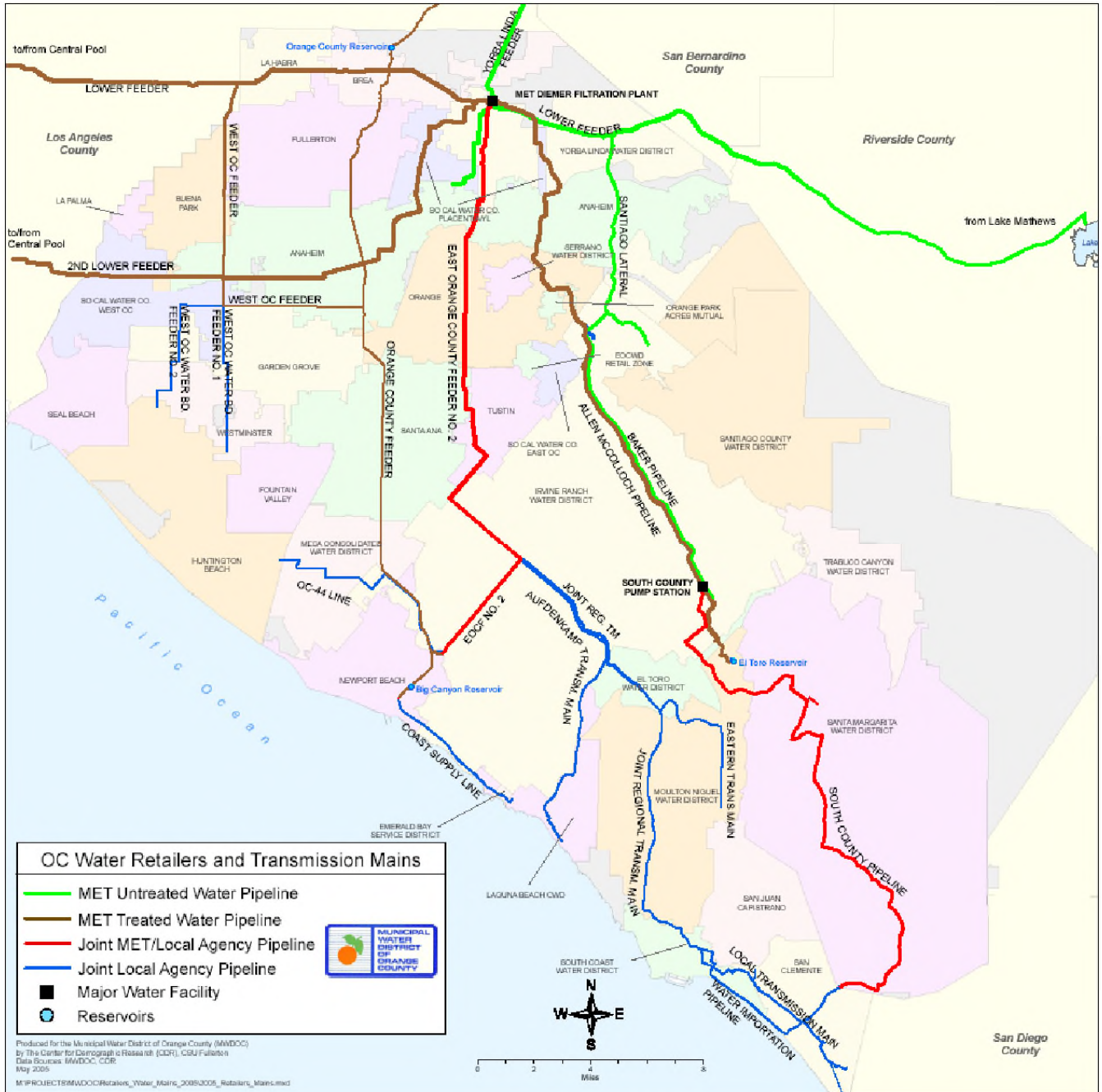
Figure 2-1: Metropolitan Feeders and Transmission Mains serving in ETWD (Municipal Water District of Orange County, 2016)
