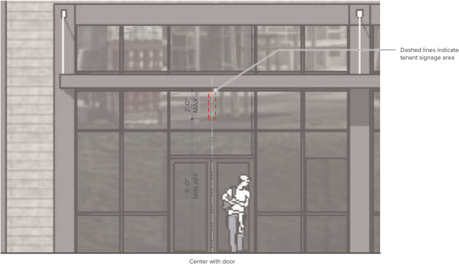
1 Example Blade Sign Elevation Scale : 1/4"=1'
