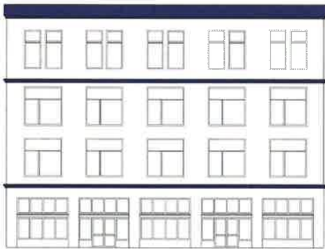
DATUM LINES ALONG THE ENTIRE LENGTH OF A BUILDING WITH CHANGE IN MATERIAL
